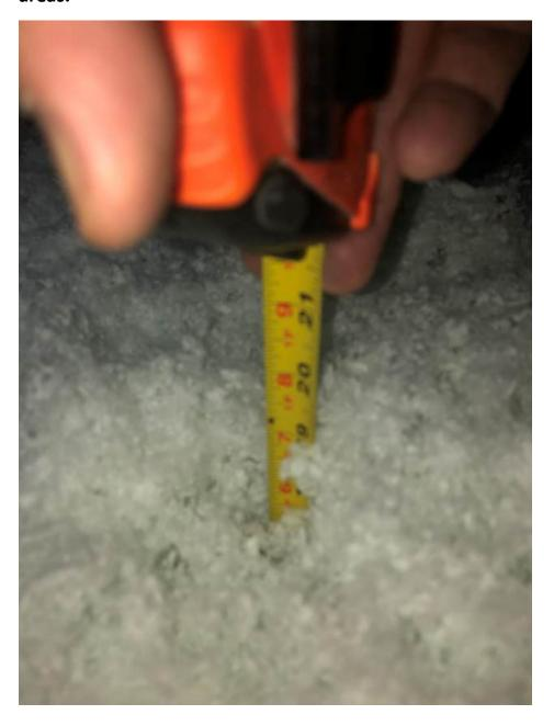
However, the insulation is a few inches low just rear of the access point in the rear attic; it should be topped up there.
